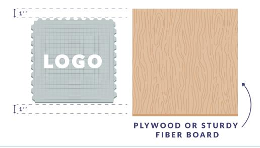
2 Slide plywood or sturdy fiberboard under the tile not allowing the rubber tile/mat to flex under the tile.
